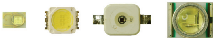
LUXEON Rebel, at far left, compared to other power LEDs.
