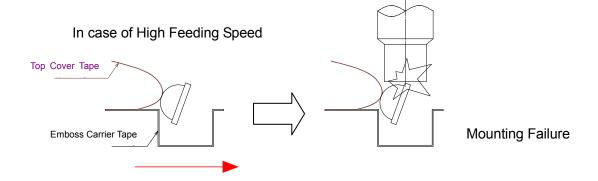
Even when the LED is in contact with the top cover tape; however, by lowering the feeding speed, it can be detached from the tape before absorbed by the nozzle.
